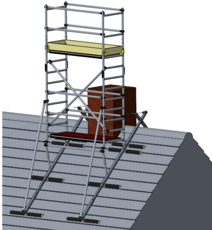
16. Finally, place the two girders between the lower eye of the two extensions and the two 8-stage frames. This provides additional stability while using the scaffolding. Should the coupling of the girder end up exactly at a rung, adjust the extension so that this problem no longer occurs.
