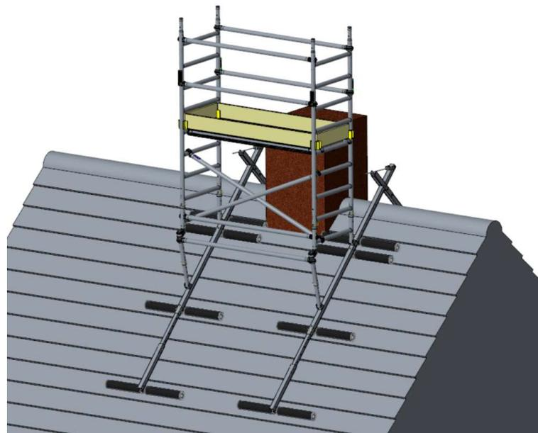
12. Place the other 4 horizontal ledgers on each side of the platform at knee and hip height. Make sure that the openings of the claws point outwards.
